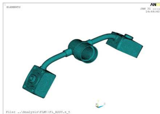
Figure 3: FEA Model of FLM.
