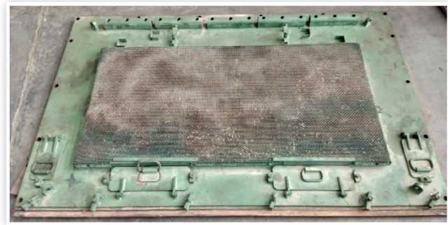
FIGURE 15 Fabricated composite cover plate for MBT
