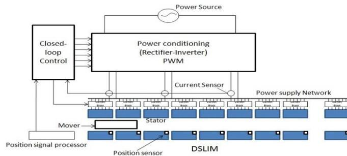
Fig. 1 The basic structure of EMALS
