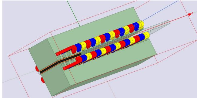
Fig. 3 3D Model of DSLIM in Maxwell
