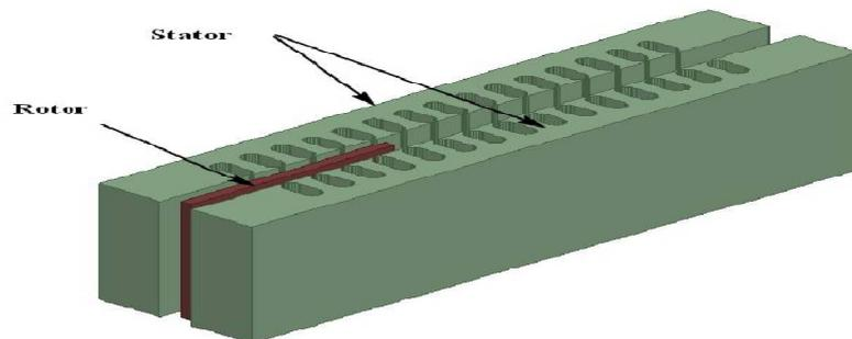
Fig. 2 DSLIM with long Stator
