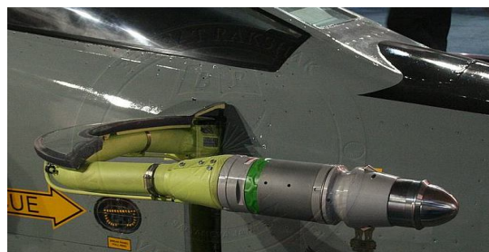
Fig. 2: Retractable/Foldable type refuelling probe
