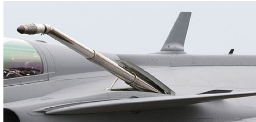
Fig. 1: Telescopic Refueling Probe
