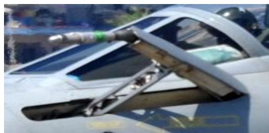
Fig. 3: Retractable/Telescopic actuated type refuelling probe
