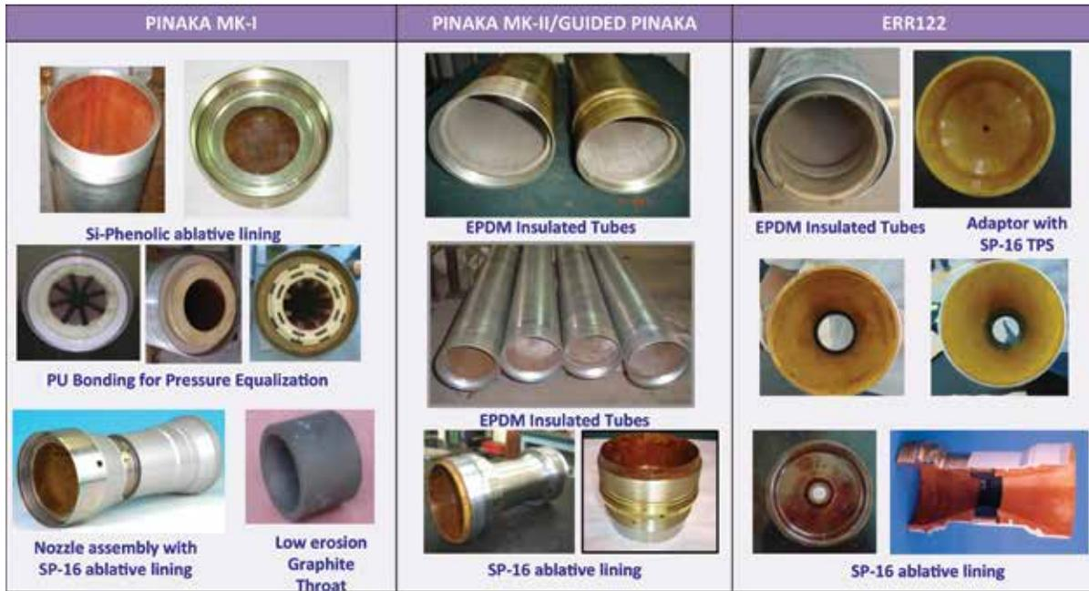
**Thermal Protection System used for Rockets**
