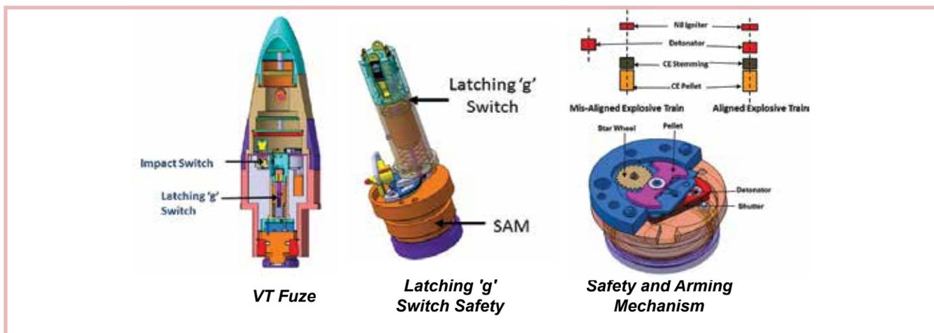
star wheel, gear, pinion and pallet mechanism. The detonator inside shutter comes to the armed position slowly. The motion of shutter is continuously hindered by the pallet and therefore it takes time (about 900 ms-1 s) for the detonator to come to aligned condition.
